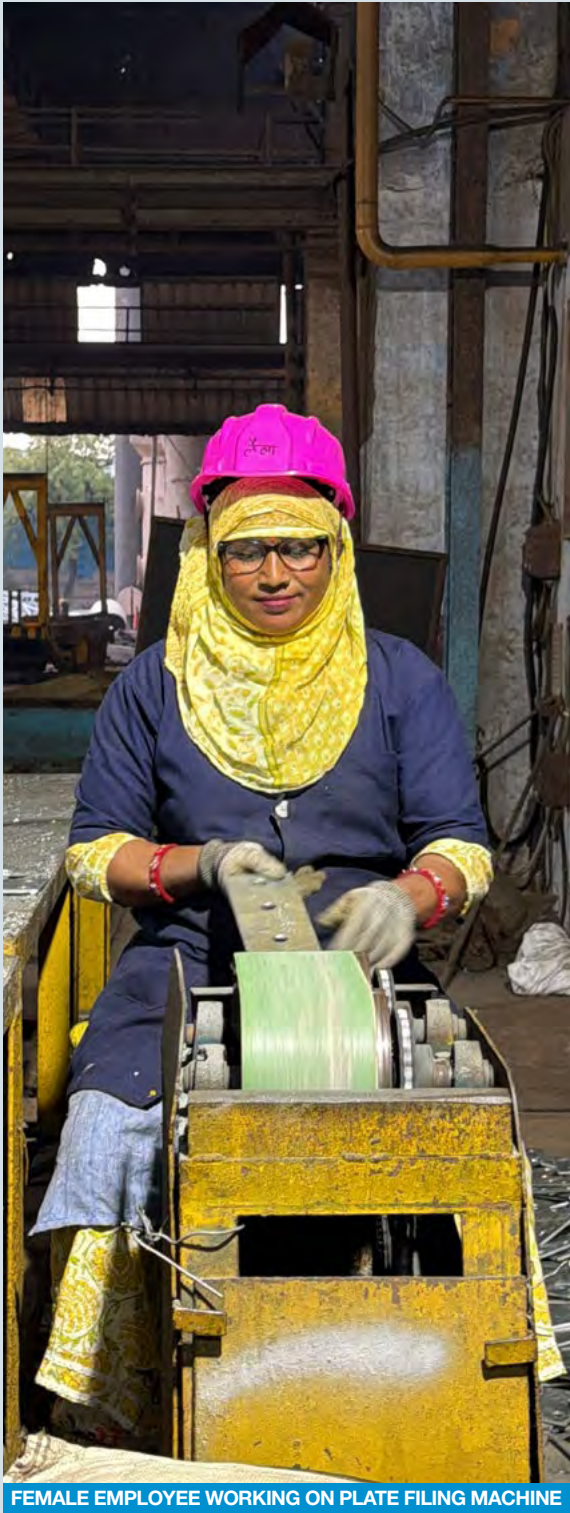
FEMALE EMPLOYEE WORKING ON PLATE FILING MACHINE
