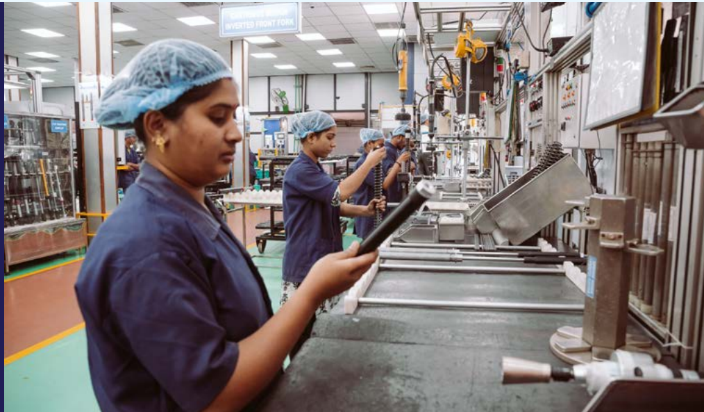
◆ Cartridge tube assembly for adjustable Inverted front fork, suspension plant, Chh. Sambhajinagar
