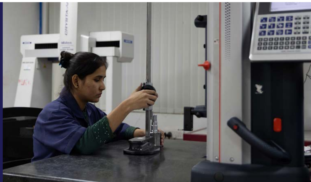
◆ Quality check on Coordinate Measuring Machine, Driveline, Waluj, Chh Sambhajinagar
