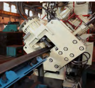
Bending - 12-metre hydraulic press brake machine from LVD (Belgium)
