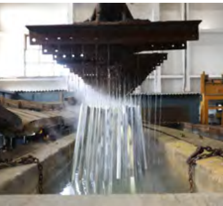
Galvanising - Remote radio-controlled hot dip galvanising plant from GIMECO, Italy
